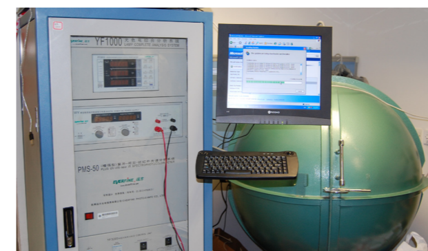
Integrated sphere for lighting measurement
