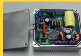
HID lamp ballast with thermal managed casing
