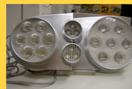
LED front lighting using 7 LEDs
