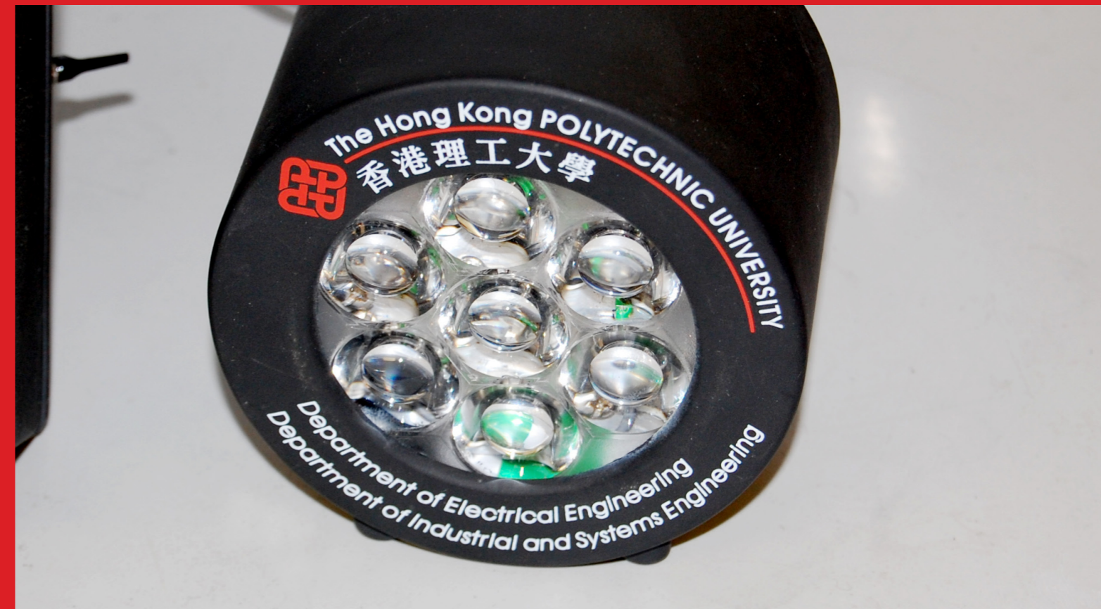
LED braking lighting using 7 superbright LEDs
